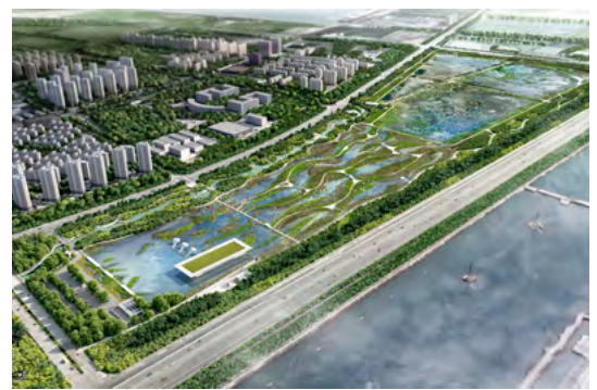
The design for Lingang Eco Park plans for wastewater recycling and rainwater harvesting, providing water to the new wetland areas.
