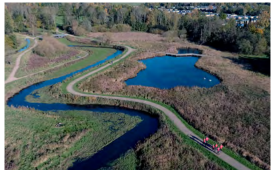
The project in Kokkedal sought to restore natural water cycles, mimicking nature and managing rainwater close to where it falls. This also provides benefits for biodiversity, recreation and landscape character.
